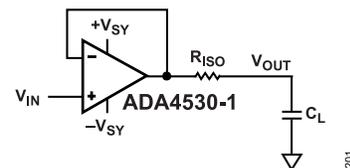
Figure 101. Stability Compensation with Isolating Resistor,  $R_{ISO}$
