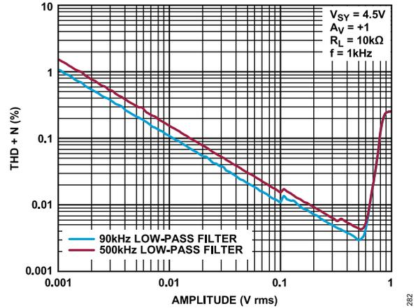
Figure 82. THD + N vs. Amplitude,  $V_{SY} = 4.5\text{ V}$
