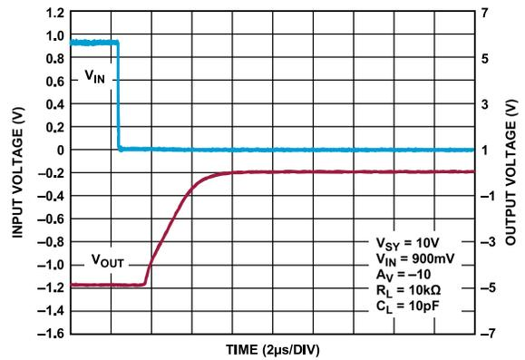
Figure 71. Negative Overload Recovery,  $V_{SY} = 10\text{ V}$
