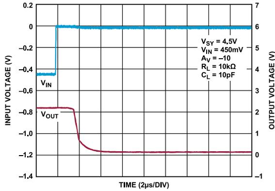
Figure 67. Positive Overload Recovery,  $V_{SY} = 4.5\text{ V}$
