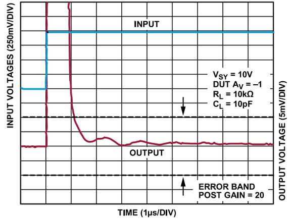
Figure 77. Positive Settling Time to 0.1%,  $V_{SY} = 10\text{ V}$
