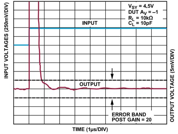
Figure 76. Positive Settling Time to 0.1%,  $V_{SY} = 4.5\text{ V}$
