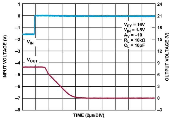
Figure 69. Positive Overload Recovery,  $V_{SY} = 16\text{ V}$
