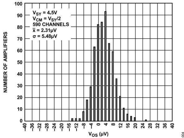
Figure 4. Input Offset Voltage Distribution,  $V_{SY} = 4.5\text{ V}$
