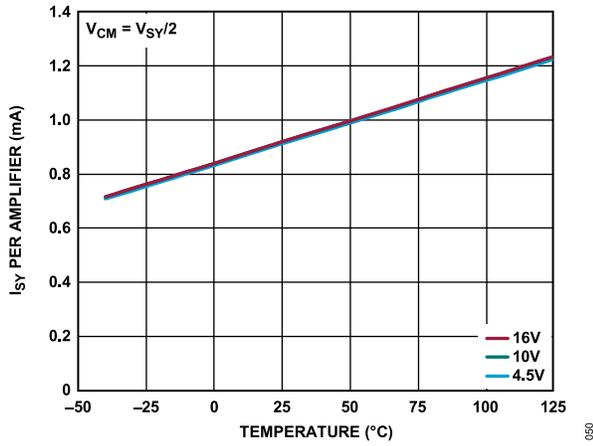
Figure 53. Supply Current ( $I_S$ ) per Amplifier vs. Temperature
