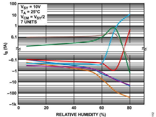
Figure 112. Effective Input Bias Current vs. Relative Humidity
