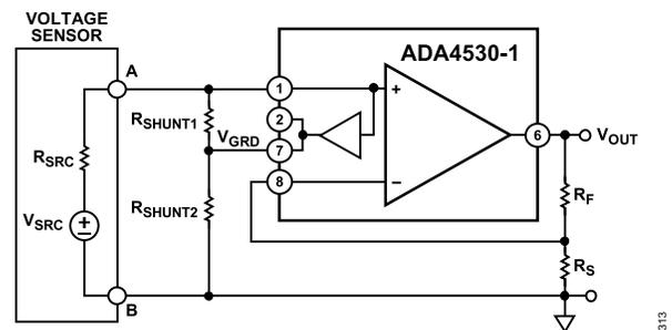
Figure 107. Voltage Buffer Circuit with Guard
