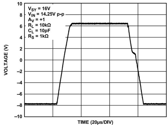
Figure 66. Large Signal Transient Response,  $V_{SY} = 16\text{ V}$
