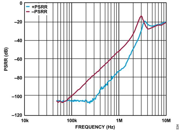
Figure 134. Positive and Negative PSRR for the ADP7118 and ADP7182 Powering ADA4530-1,  $\pm V_{SY} = \pm 5$  V,  $+IN = 0$  V
