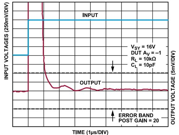
Figure 78. Positive Settling Time to 0.1%,  $V_{SY} = 16\text{ V}$
