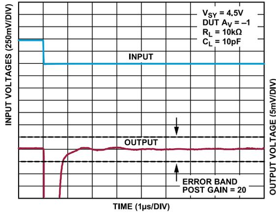
Figure 73. Negative Settling Time to 0.1%,  $V_{SY} = 4.5\text{ V}$
