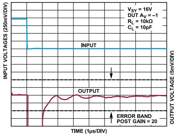
Figure 75. Negative Settling Time to 0.1%,  $V_{SY} = 16\text{ V}$
