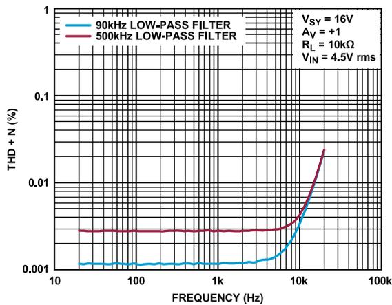
Figure 81. THD + N vs. Frequency,  $V_{SY} = 16\text{ V}$
