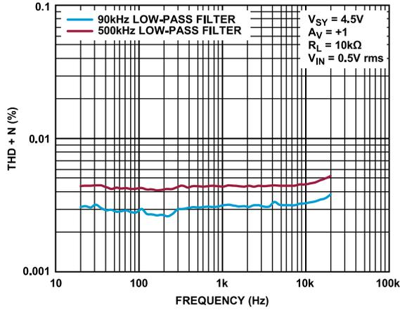
Figure 79. THD + N vs. Frequency,  $V_{SY} = 4.5\text{ V}$
