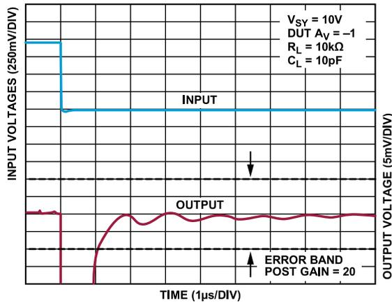
Figure 74. Negative Settling Time to 0.1%,  $V_{SY} = 10\text{ V}$
