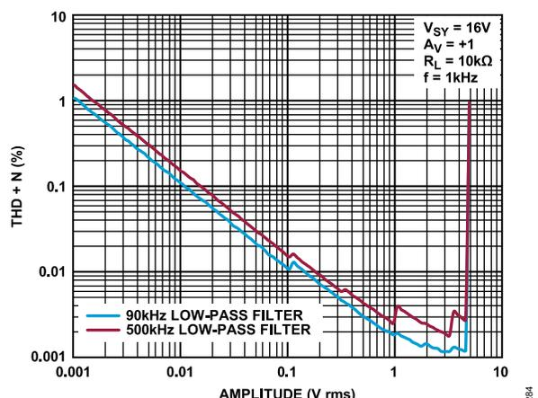
Figure 84. THD + N vs. Amplitude,  $V_{SY} = 16\text{ V}$
