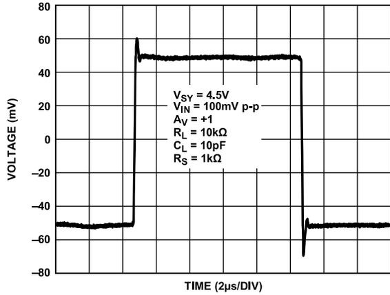
Figure 61. Small Signal Transient Response,  $V_{SY} = 4.5\text{ V}$
