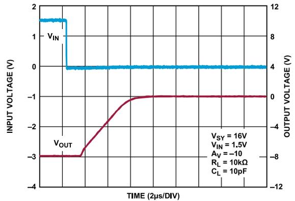
Figure 72. Negative Overload Recovery,  $V_{SY} = 16\text{ V}$
