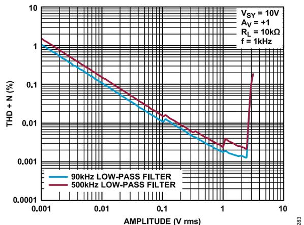
Figure 83. THD + N vs. Amplitude,  $V_{SY} = 10\text{ V}$
