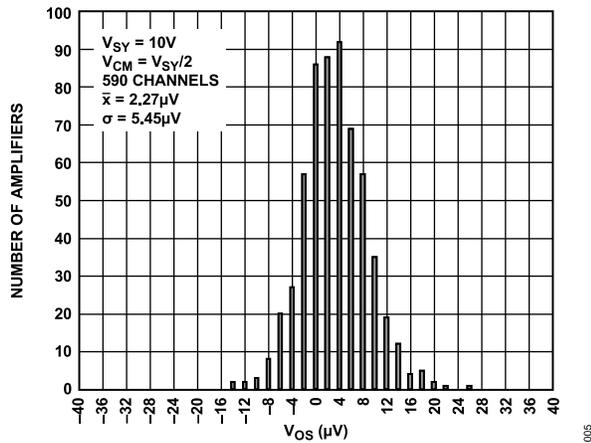
Figure 5. Input Offset Voltage Distribution,  $V_{SY} = 10\text{ V}$
