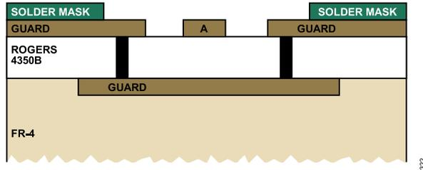
Figure 123. Layout Cross Section with Guard Plane
