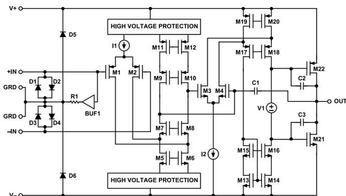
Figure 99. Simplified Schematic
