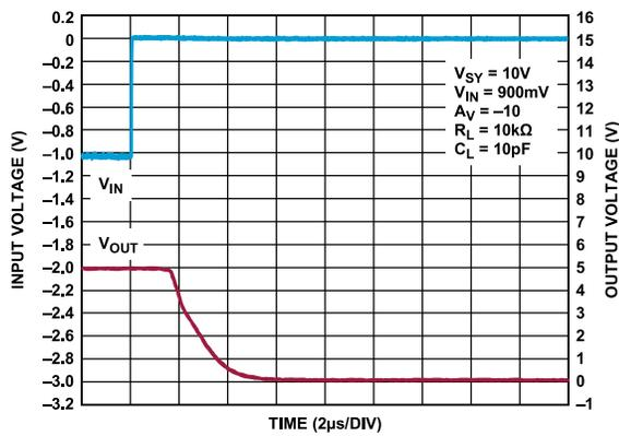
Figure 68. Positive Overload Recovery,  $V_{SY} = 10\text{ V}$
