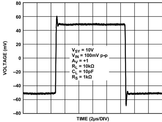
Figure 62. Small Signal Transient Response,  $V_{SY} = 10\text{ V}$
