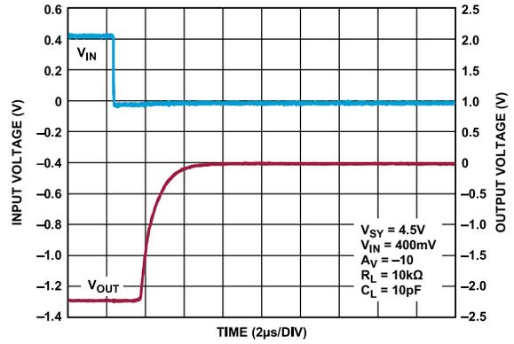
Figure 70. Negative Overload Recovery,  $V_{SY} = 4.5\text{ V}$
