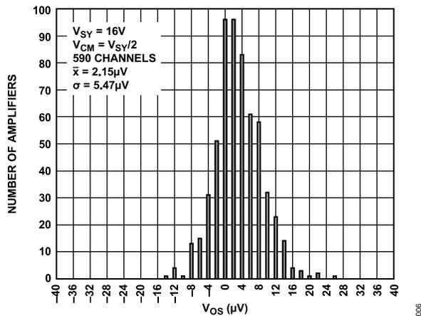
Figure 6. Input Offset Voltage Distribution,  $V_{SY} = 16\text{ V}$
