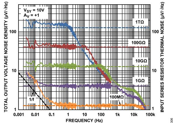
**Figure 117. Transimpedance NSD Referred to Output**
