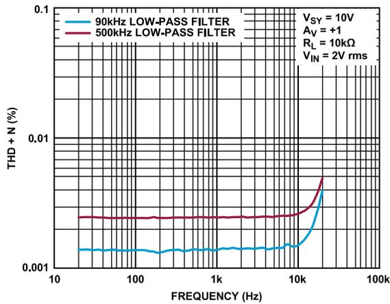
Figure 80. THD + N vs. Frequency,  $V_{SY} = 10\text{ V}$
