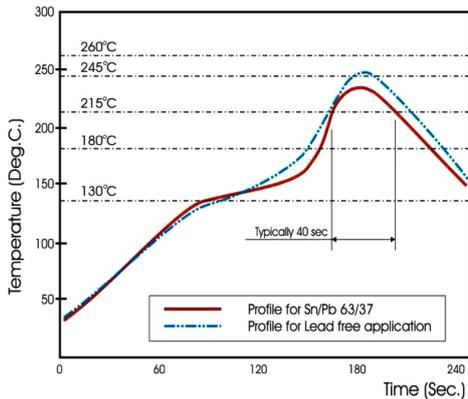
**Infrared soldering profile for Chip Resistors
