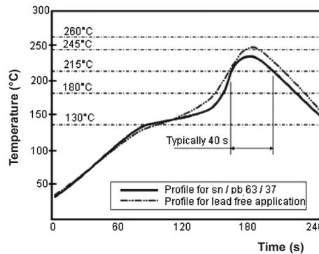
Infrared soldering profile for Chip Resistors
