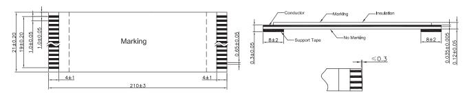
Dimensions: Millimetres Tolerances: ±0.3mm
