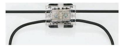
Housing material: polycarbonate trasparent Self-extinguishing: UL 94 - V0; IEC 695-2-1 a 850 °C; IEC 695-2-2 Exercice temperature: T 85 °C Clamps: Brass nickel plated Screws: Galvanized steel Voltage rating: 450 V Voltage test: 2500 V Protection degree: IP 20 According noms: CEI EN 60998-1 1995 CEI EN 60998-2-1 1995 CEI EN 60999-1994 CEI EN 60947-7-1 1992
