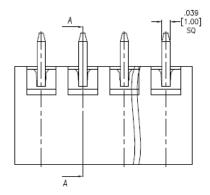
Positions: 02 thru 24 A = .200 [5.08] x No. of Positions + .055 [1.40] B = .200 [5.08] x No. of Spaces
