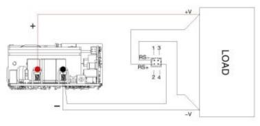
Remote sensing function wiring diagram
