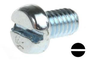
Cheese Head Machine Screws are designed for ease of assembly and these screws with their slotted drives are a popular driving method with this type of fastener. Machine screws can be used in pre-tapped holes or used with conforming nuts and washers in through-holes.
