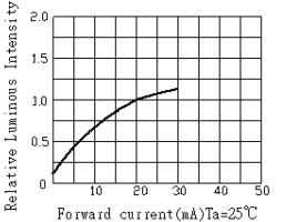
Luminous Intensity vs.Forward current
