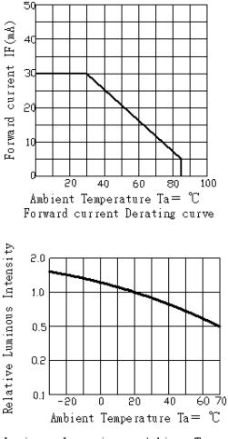
Luminous Intensity vs.Ambient Temperature
