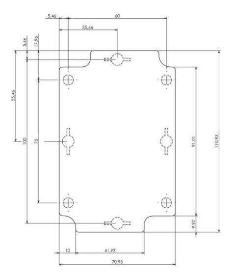
Dashed line shows outline of the mounting boss under PCB board Recommended mounting holes diameter ø4mm
