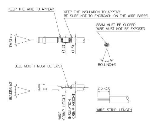
Wire Crimp Information for MP-565-290-721-P60 Contact with Insulation DIA 1mm to 1.3mm.
