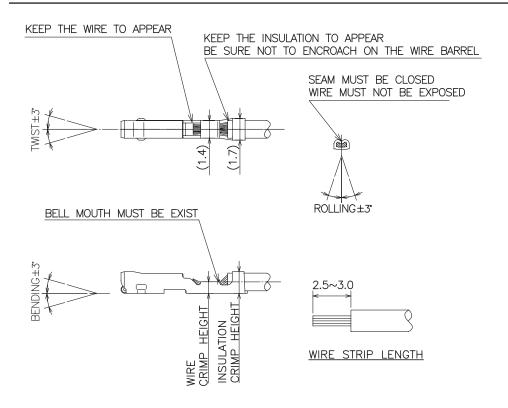
Wire Crimp Information for MP-565-290-741-P60 Contact with Insulation DIA 1.3mm to 1.7mm.
