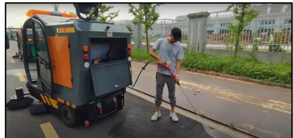
In-built High Pressure Washing System
