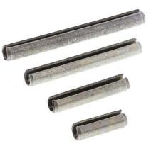
Slotted Spring Pins consist of a single coil of spring steel with an open slot which enables the pin to reduce in diameter as it is driven into a hole of appropriate size.
