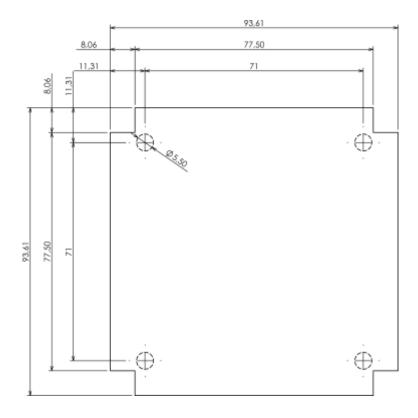
Dashed line shows outline of the mounting boss under PCB board Recommended mounting holes diameter Ø3.5 mm All dimensions are given within +/-0,5mm tolerance
