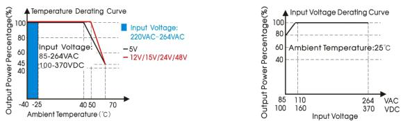
Note: ① With an AC input between 85-110VAC and a DC input between 100-160VDC, the output power must be derated as per temperature derating curves; 2) This product is suitable for applications using natural air cooling; for applications in closed environment please consult factory or one of our FAE.
