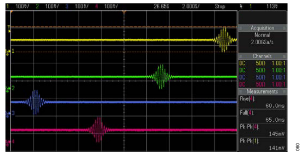
Figure 59. Programming Example 5: Four Pulsed DDS-Generated Sine Waves Amplitude modulated by an SRAM Vector with Different Start Delay
