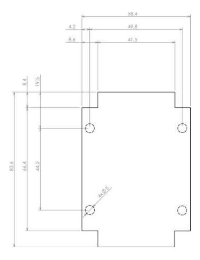
Dashed line shows outline of the mounting boss under PCB board Recommended mounting holes diameter  $\emptyset 3,5 \mathrm{mm}$
