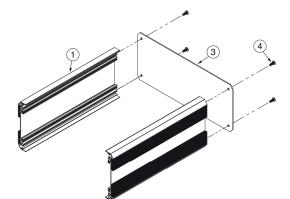
Install ③ front/rear panel to ① side frame and secure with ④ Umbrella Phillips Screw M5-10 (Dog Point).
