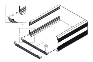
Install (6) GP Bar Kit [option] into the slide rail slot in side frame and secure with GP Bar position by Umbrella Phillips Screw M5-10 (Dog Point). We advise to install user components at this stage. Our GP Bar Kits are ideal for this purpose, but user can prepare their own method.
