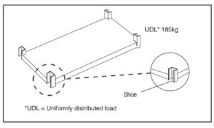
The base unit is used to hold the uprights or CV (Centrafour Vertical). The base unit also helps maintain the bay dimensions, acts as a lower storage level and is integral to the overall strength of the unit.
