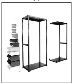
The basic and additional bays shown above must not have a combined UDL (uniformly distributed load) that exceeds 945kg. Therefore each bay must not exceed 945kg and the shelves must not individually exceed 135kg UDL.
