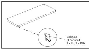
Shelves are manufactured in cold reduced steel CR4 to BS 1449 part 1, are 1.0m wide and 500mm deep. They have a thickness of 20swg and are available in a light grey stove enamel finish.
