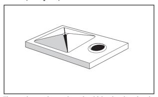
The packer or base plate should be fitted under the upright or CV to spread the load and prevent the section punching into the floor. Manufactured from 2.6mm CR4 steel.
