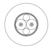
Cable Marking: RS PRO 2 Core×0.22mm<sup>2</sup>
