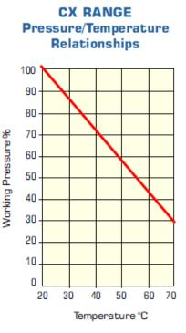
Max. recommended continuous working temperature =  $60^{\circ}C$
