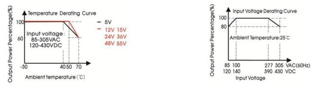
Note: 1.With an AC input voltage between 85-100VAC and a DC input between 120-140VDC the output power must be derated as per the temperature derating curves;
