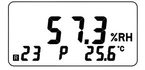
⇒ Press "MEMORY" momentarily to decrease the displayed record by 10, continuing to press the "MEMORY" button momentarily will cycle the readings continually.
