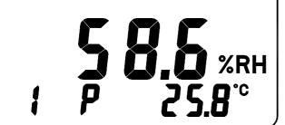
⇒ The number of memorized records increases by 1 to the maximum of readings of 99.
