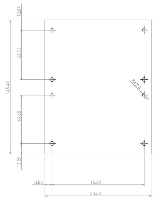
Dashed line shows outline of the mounting boss under PCB board Recommended mounting holes diameter ø3,5mm
