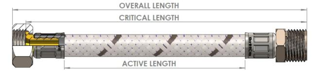
Critical length is the distance between hose mating faces. This must be 10% greater than the actual distance between the two corresponding fixed mating parts to avoid tensile stress whilst in service.
