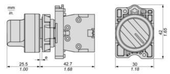
(e) Clamping thickness: 1 to 6 mm / 0.04 to 0.24 in.
