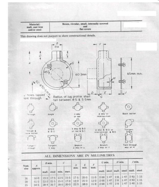
NOTE. Dimension G applies to unmachined parts only.
