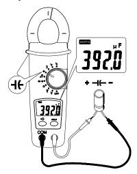
Note – To improve the measurement accuracy of a small value capacitor, record the reading with the test leads open circuit, then substract the residual capacitance of the Instrument and leads from the final measurement.
