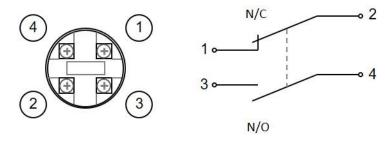
The switch is not polarity sensitive
