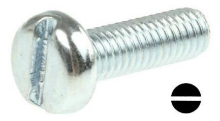
Pan Head machine screws, similarly to Oval Head machine screws have rounded sides, however the difference being that Pan Head machine screws have a flat top rather than a rounded one. The slotted drive is a popular driving method with this type of fastener for ease of assembly. Machine screws can be use din pre-tapped holes or used with conforming nuts and washers in through holes.
