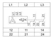
L1,L2,L3 : Supply to be monitored 11-14,12 : 1st C/O contact of output relay 21-24,22 : 2nd C/O contact of output relay
