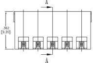
Positions: 02 thru 24 A= .138 [3.50]  $\times$  No. of Spaces + .169 [4.30] B= .138 [3.50]  $\times$  No. of Spaces
