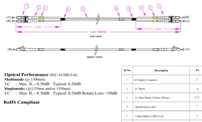
Connector: LC clips shall be mounted on to the connector to make it duplex.
