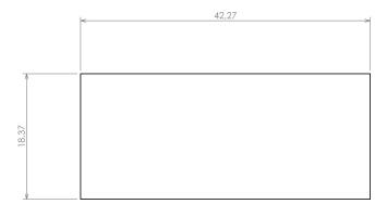
Dashed line shows outline of the mounting boss under PCB board Recommended mounting holes diameter ø3,5mm All dimensions are given within +/-0,5mm tolerance
