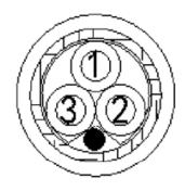
Cable Marking: RS PRO 3 Core×0.25mm<sup>2</sup> Screened Industrial Cable 250V
