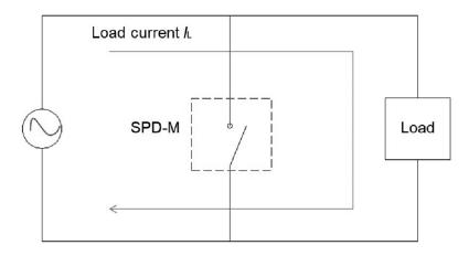
When a surge invades the circuit, the SPD-M circuit mutates to a low impedance, releasing the surge current into the ground
