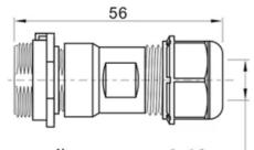
Cable outer diameter range: 6-10mm
