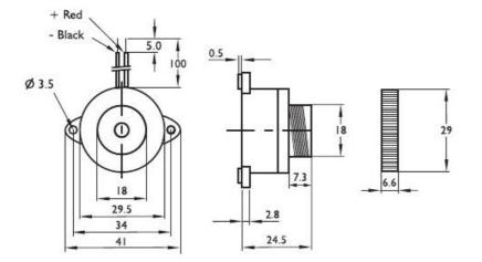
Dimensions Unit: mm Tolerance: ±0.5mm
