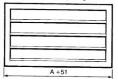
Louvres are manufactured in one piece units up to 1800mm square.
