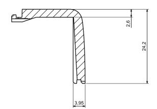
All dimensions are given within +/-0,5mm tolerance
