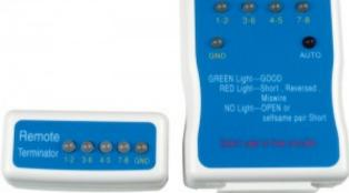
This basic level network tester will comprehensively test each twisted pair through RJ45 or RJ11 connectors. An easy red and green light system will notify you of which pairs are fully functional and which are faulty. Comes with remote end terminator for testing links and patchcords. Requires 1X 9V battery (not included).
