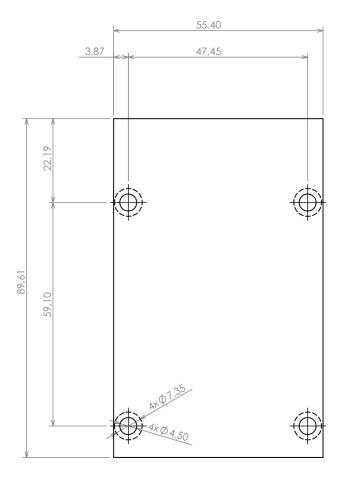
Dashed line shows outline of the mounting boss under PCB board Recommended mounting holes diameter ø3,5mm All dimensions are given within +/-0,5mm tolerance
