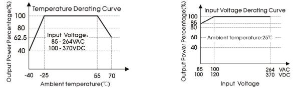
Note: ① With an AC input between 85-100VAC and a DC input between 100-120VDC, the output power must be derated as per temperature derating curves; (2) This product is suitable for applications using natural air cooling; for applications in closed environment please consult factory or one of our FAE.
