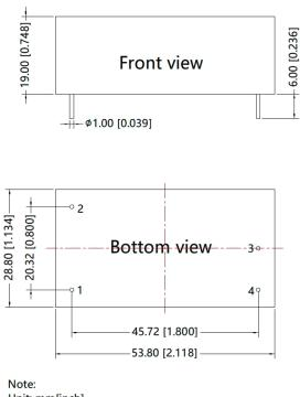
Unit: mm[inch] Pin diameter tolerances: ±0.10[±0.004] General tolerances: ±0.50[±0.020]
