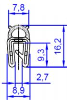
Clamping Range 1-2mm Black EPDM 60 ±5 Shore, Including Looped Wire Carrier & Hollow Sponge Sealing Section
