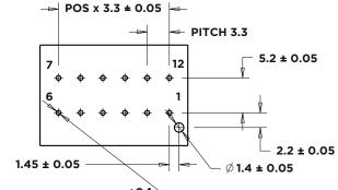
PUNCHED HOLE : Ø 0.7 +0.1 ≥ DRILLED HOLE: 0.8 ± 0.05
