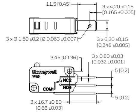
**FIGURE 8. V19 SERIES E-STYLE QUICK CONNECT •**
