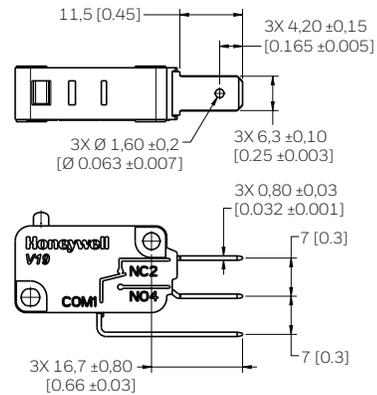
**FIGURE 10. V19 SERIES P-STYLE STRAIGHT PCB TERMINAL**
