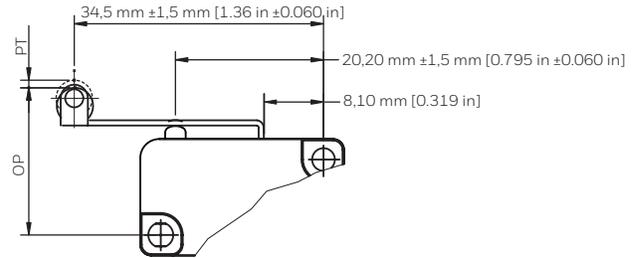
NOTE: These dimensions apply for the "A" lever position. For the "B" lever position, please add 5,8 mm [0,224 in].
