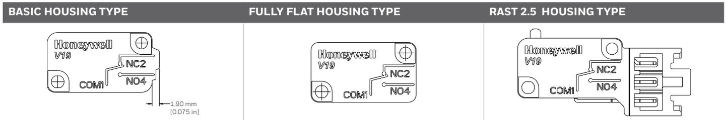
FIGURE 5. V19 SERIES RAST 2.5 SWITCH DIMENSIONS
