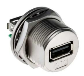
The RS PRO series of waterproof metal USB-A connectors are a range of ruggedised IP67/IP68 connectors designed to be used outdoors or in harsher industrial environments. Designed to fit panel cut outs of 25.5mm the metal USB-A series also comes with rear potting on the panel mount connectors. This ensures your panel is still sealed to an IP67/IP68 rating even when the connector is unmated, and the sealing cap is not connected. The threaded mating allows for a secure connection.
