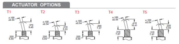
NONE: T1,T2,T3 Actuator shown with B1 to B4 bushing, subtract 0.09 ( 2.29 ) for B5 bushing, subtract 0.04 ( 1.02 ) for B7 bushing. T4,T5 Actuator shown with B5,B6 bushing, add 0.09 ( 2.29 ) for B1 to B3 bushing, add 0.05 ( 1.27 ) for B7 bushing. Std for M1,M2 Terminal sub .016(.040) for M6,M7,VSX
