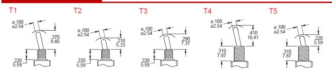
NONE: T1,T2,T3 Actuator shown with B1 to B4 bushing, subtract 0.09 ( 2.29 ) for B5 bushing, subtract 0.04 ( 1.02 ) for B7 bushing. T4,T5 Actuator shown with B5,B6 bushing, add 0.09 ( 2.29 ) for B1 to B3 bushing, add 0.05 ( 1.27 ) for B7 bushing. Std for M1,M2 Terminal sub .016(.040) for M6,M7,VSX
