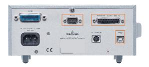
With respect to connecting the external control, RM-804/805 provide a D-sub 25-pin composite interface to execute, according to the functionalities, Handler, Scan or EXT IO for connecting to a sorting machine; connecting to an external on-off switch, and directly conducting external trigger control
